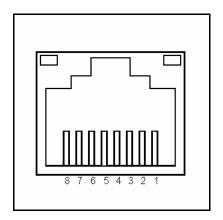
Figure 14 - RJ45 Ethernet port pin-out
